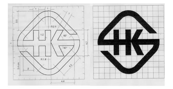
The Hong Kong Safety Mark may appear in any size provided it is not less than 5mm in height. The Mark can be enlarged or reduced with its aspect ratio remaining unchanged. Where limitations of space prevent the use of the Mark in the minimum size (i.e. 5mm in height), requests to use a Mark of smaller dimensions will be considered by HKCC on the basis of legibility.
